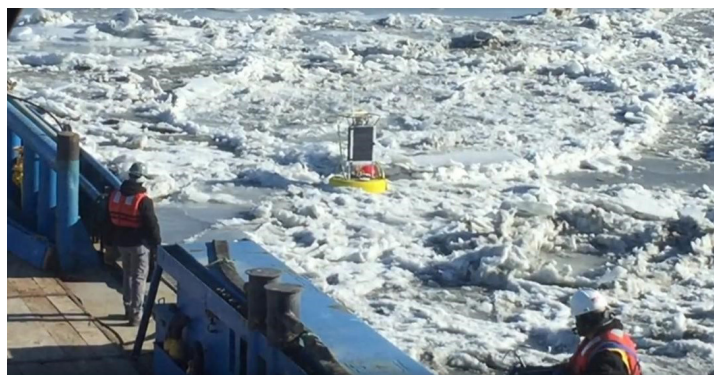
Figure 4. Aridea buoy-based monitoring system with Aqua TROLL 600.
